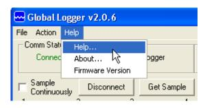
**COM Status:** This reads "Connected" in green or "Not Connected" in red, depending on the current connection status.
