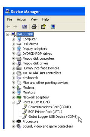
8) To confirm the installation, look in the Device Manager and find the USB Serial Port. The COM setting following that will show the virtual COM port that has been automatically assigned to the driver. As you will see in the following sections, this COM port will be automatically detected by the Global Logger software so it is not necessary to note which port is being used by the driver.
