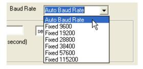
you must set the baud rate in the opening connection menu of the Global Logger II software to this speed, or the logger will not communicate.
